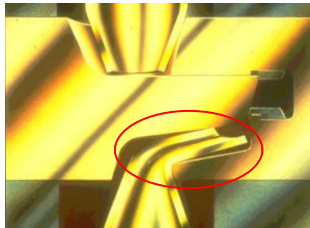
Figure 3.5 – Cameron SBR or DVS rams with drill pipe folded over.
