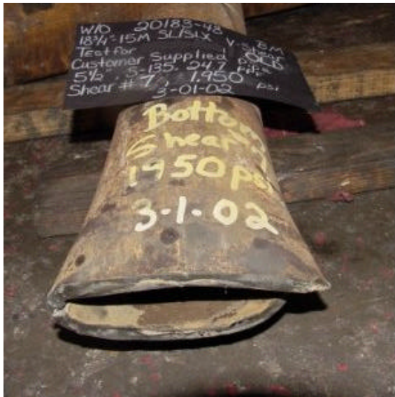
Figures 3.1 and 3.2: Example shears of low ductility or brittle pipe (left) and high ductility pipe (right). The high ductility pipe required almost 2,000 psi (over 300,000 lb) more to shear than the low ductility pipe even though the grades on both pipes were the same, S-135. Visual differences in the shears can also be easily noted: the brittle pipe on the left has cracking on the sides and did not collapse as much as the more ductile pipe on the right. The ductile pipe had no cracking on the sides. In the severest of cases, very brittle pipe cracks considerably when being collapsed by the shear rams and then requires less force to complete the shear.
